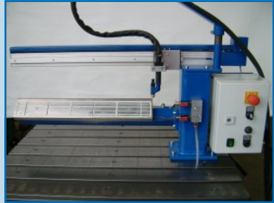
welding of corner joints onto vacuum beam
