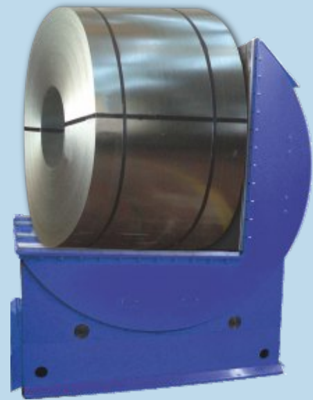
rotary jig / coil turner for heavy loads up to 40 t
