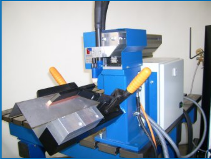
mechanized longitudinal seam welding
