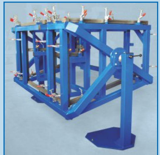
Welding jigs for big 3D-components
